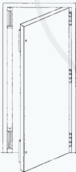
Fig. 6 Single door. Double lock mounted vertically with full length housing. Note: Check baskset dimension when using latching hardware. (E08551)
